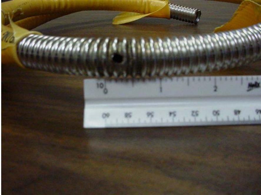
Figure 1 Typical Lightning Damage to CSST
